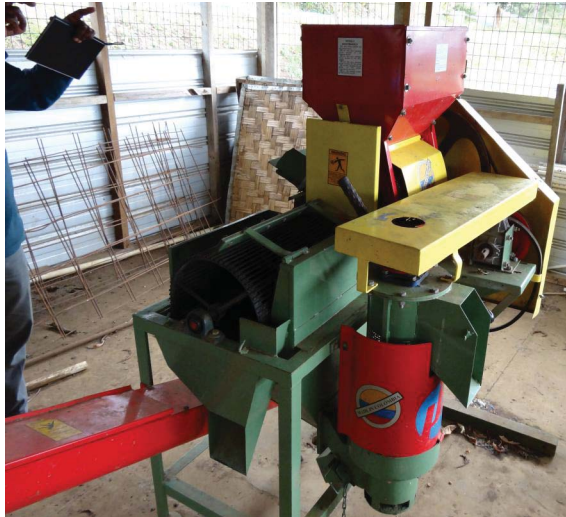
Plate 10.4 Penagos ecopulper : combined drum pulper linked to demucilager
